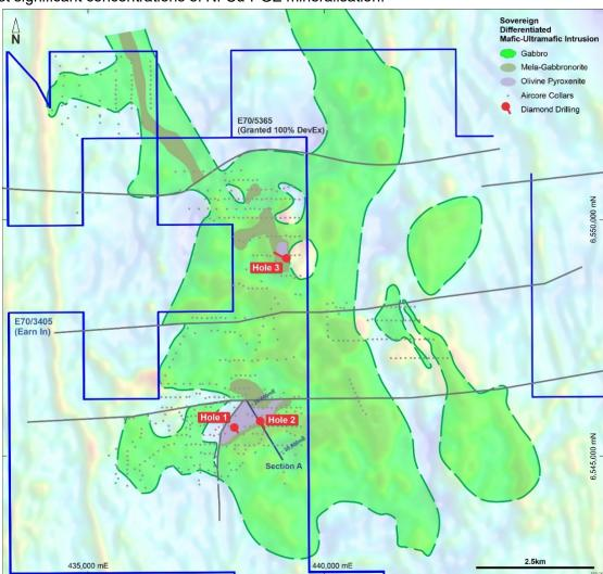
**Figure 1.** Sovereign Project: Location of three diamond drill holes 21SVDD01 (Hole 1) - 21SVDD03 (Hole 3), drilled to understand the local geology and framework of the mafic ultramafic intrusion. Local grid provided for context to Figure 2.
