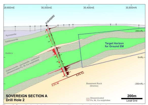
**Figure 2.** Generalised geological cross section and interpretation with nickel and copper assays represented as histograms (Oblique to GDA Grid – temporary local grid provided – see Figure 1) showing distribution of low grade disseminated nickel-copper sulphide mineralisation within and at the base of the mafic-ultramafic intrusion. Shallowing position of these zones provides a focus for Ground EM in January 2022.
