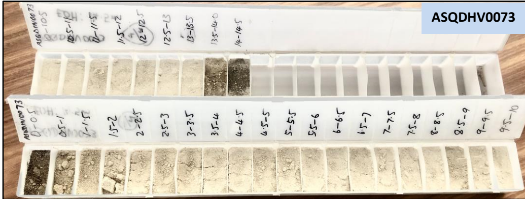
Figure 4: Vacuum drill hole ASQDHV0073 sample tray showing silica sand intersection from 0.5-13.5 m
