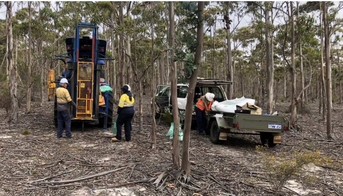
Vacuum drilling by ASQG of silica sand in a tree farm at the Albany White Hill Silica Sand Project
