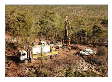
2023 RC Drilling at Quartz Hill
