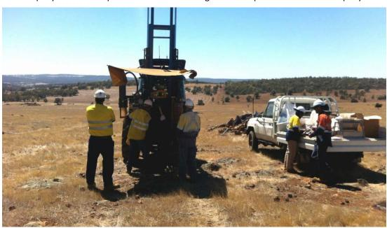
BRL drilling rig operating on cleared private farmland with bauxite outcropping at surface.
