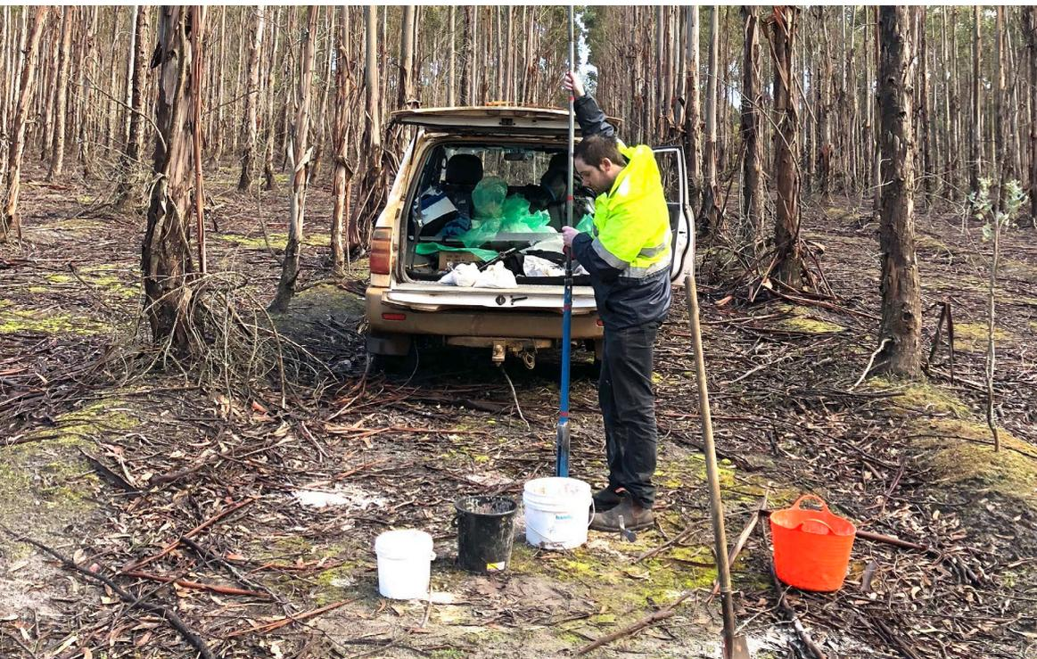
*Hand auger drilling by ASQG of silica sand in a tree farm at the Albany White Hill Silica Sand Project*
