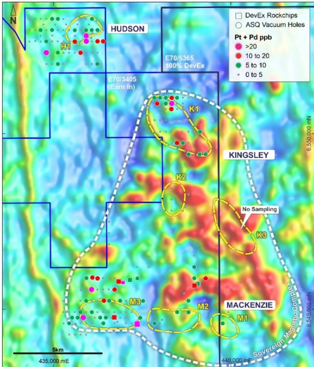
**Figure 2:** Sovereign Magnetic Complex, showing airborne magnetics (RTP) and location of airborne electromagnetic targets (yellow outlines) with **Pt+Pd** analysis of pulps from previous bauxite drilling and rock chip samples.
