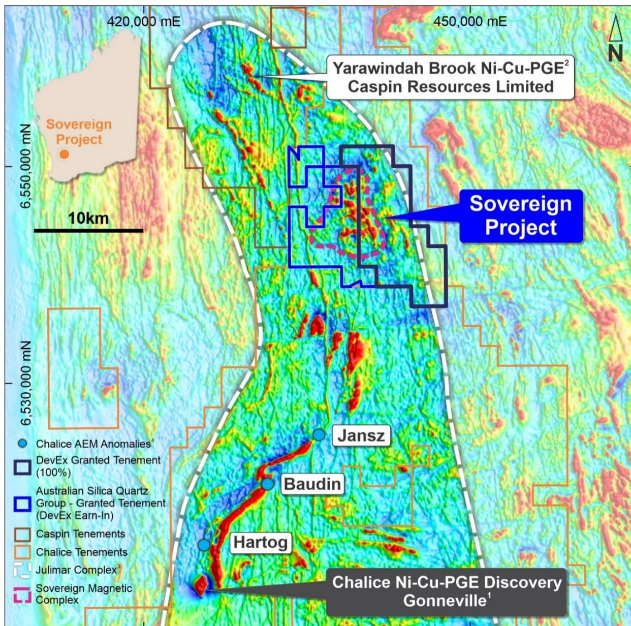
**Figure 1.** DevEx tenement application and the Australian Silica Quartz Group Ltd ('ASQ') tenement overlying airborne magnetics (RTP) in relation to Chalice Mining Limited's recent high-grade palladium-nickel discovery (ASX: CHN) at the Julimar Project.
