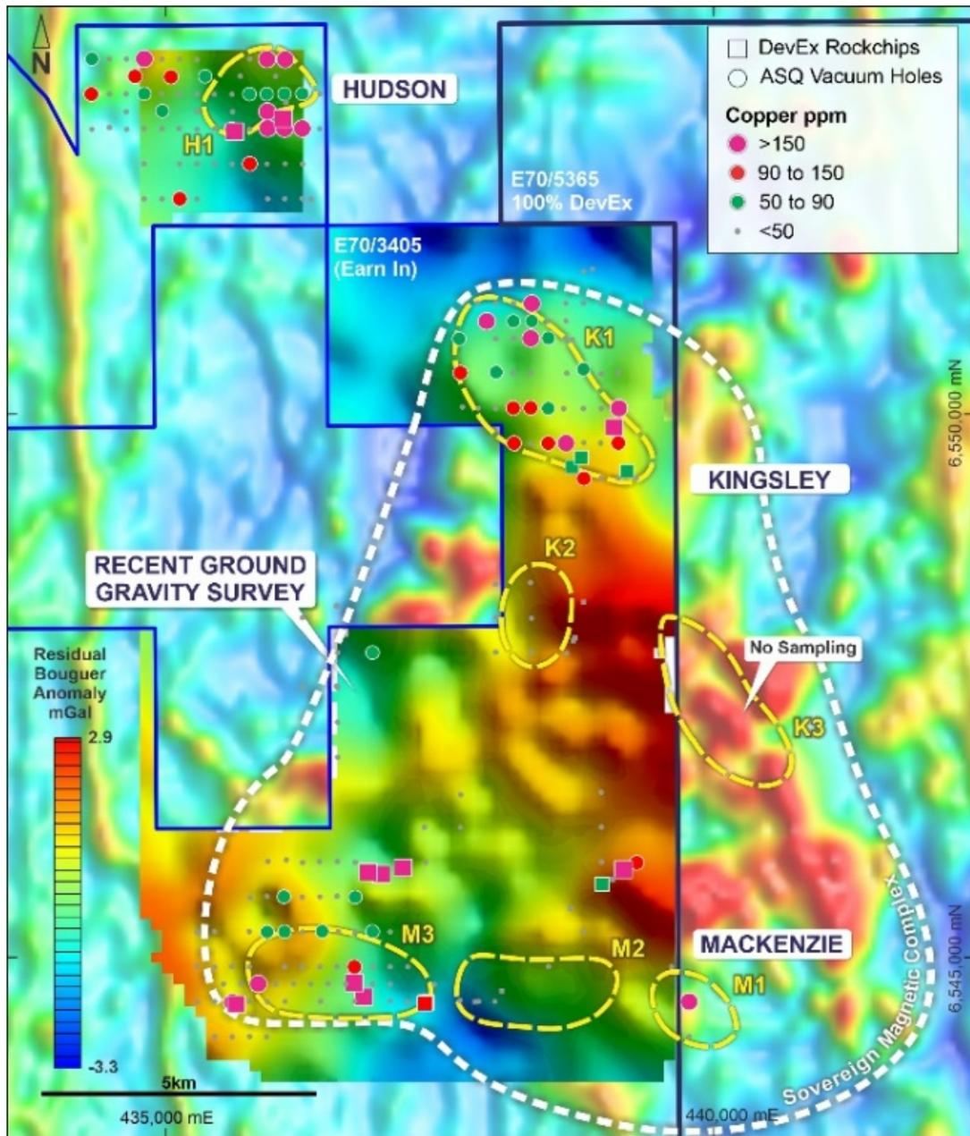
**Figure 3:** Ground gravity (Residual Bouguer) over airborne magnetics (RTP) and location of airborne electromagnetic targets (yellow outlines) with Cu analysis of pulps from previous bauxite drilling and rock chip samples.
