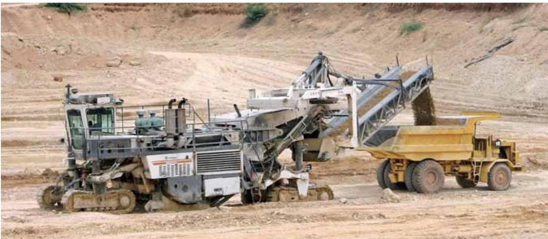
*Continuous Surface Bauxite Mining; strips, crushes and loads in one process.*
