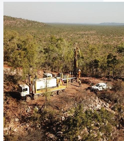
RC drilling underway at Quartz Hill
