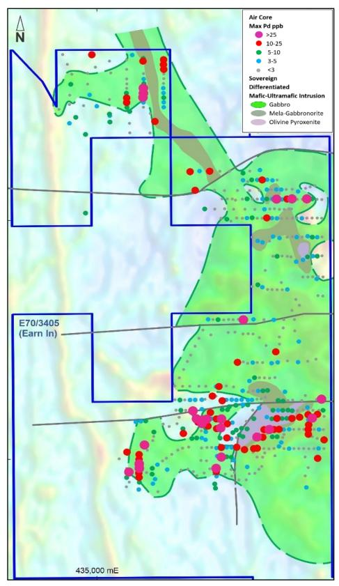
*Figure 3: Sovereign Project air-core drilling on E70/3405 with the outline of the mafic/ultramafic intrusion interpreted by DevEx from drilling results and magnetics.*
